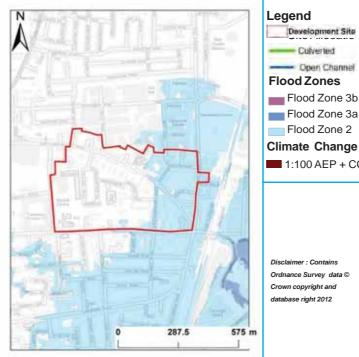
Legend Development Site Culverted Open Channel Flood Zones Flood Zone 3b Flood Zone 3a Flood Zone 2
