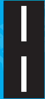
Hazard warning line
