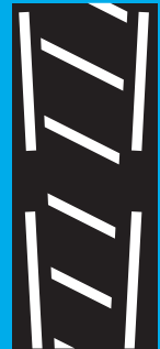
Do not enter marked area unless it is safe to do so
