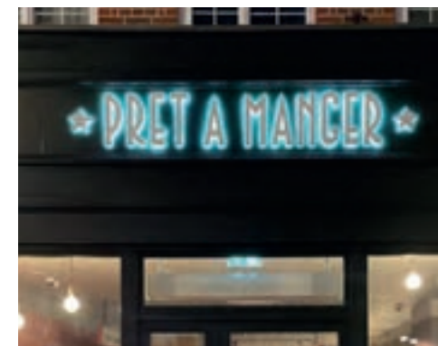
Halo lighting to individual letters may be appropriate in some instances, with lights placed behind the lettering and projecting onto the fascia, reducing glare.
