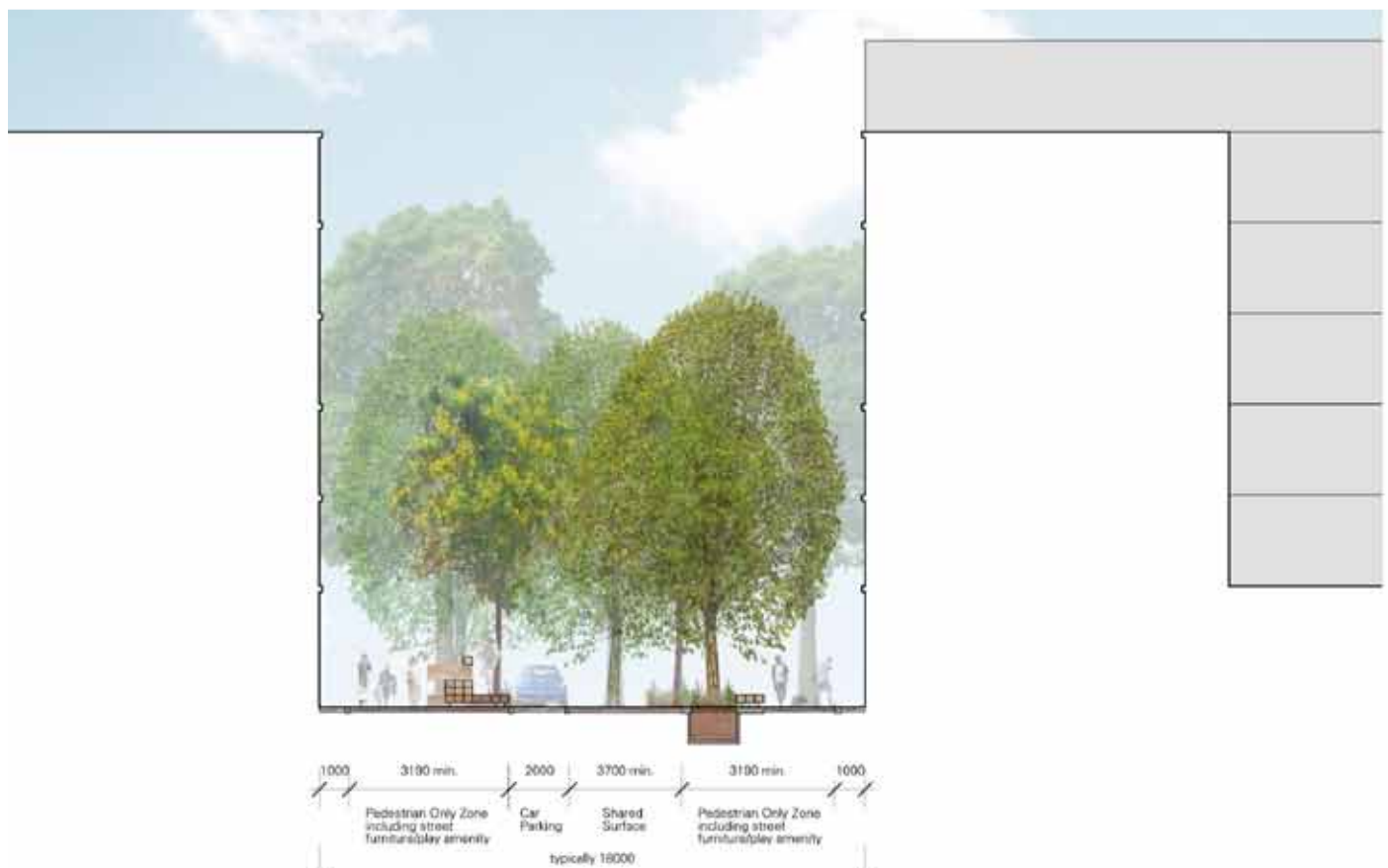
Section through Green Finger looking west
