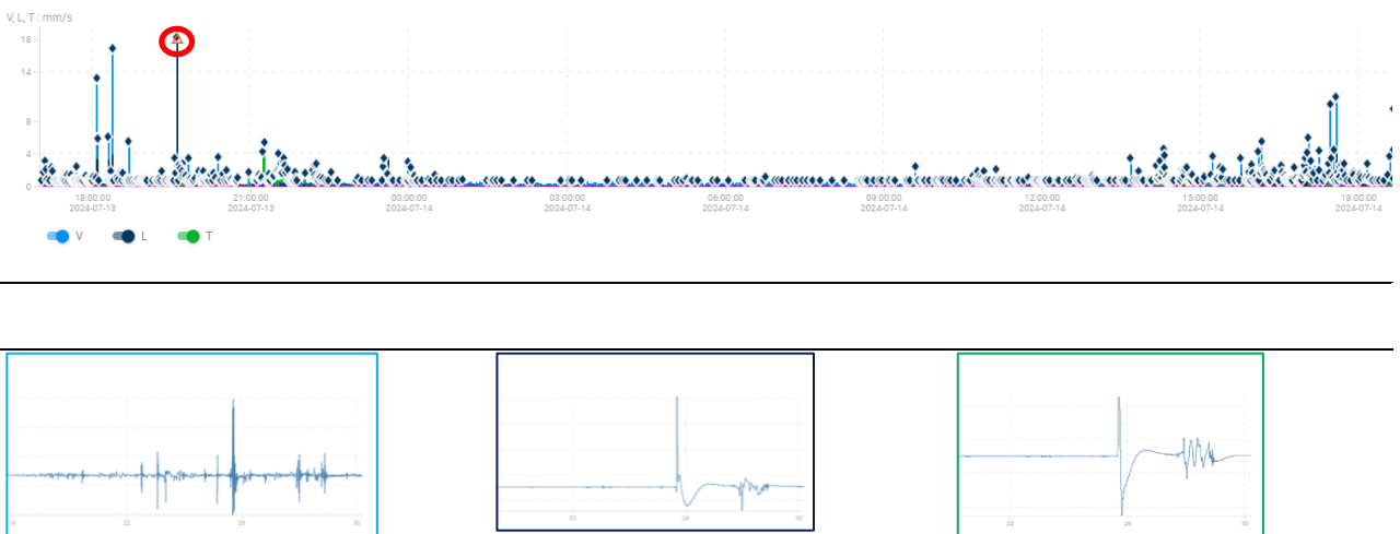
Figure 6 Foxglove Court overview of vibration. Highest amplitude vibration event axial components highlighted (Bottom left – V axis, Bottom middle – L axis, Bottom right – T axis).
