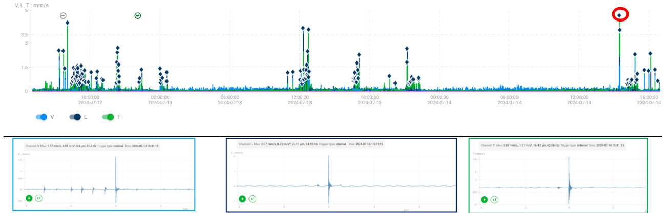
Figure 8 Park House overview of vibration. Highest amplitude vibration event axial components highlighted (V axis – bottom left top, L axis – bottom middle & T axis – bottom right).
