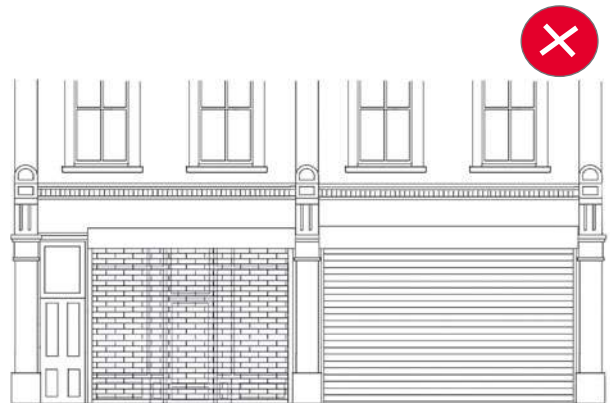
Picture 23. External Roller shutters are not appropriate.
