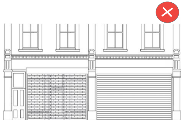
Picture 37. External Roller shutters are not appropriate.
